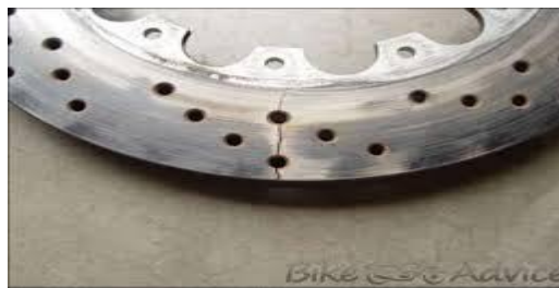
Scarring of Disc Rotor [4]
