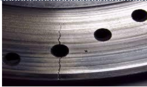
Fig. Cracking of Disc Rotor [4]
